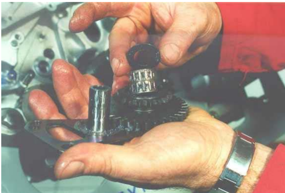
Rear cylinder timing gear (operated by crankshaft) - clutch side
